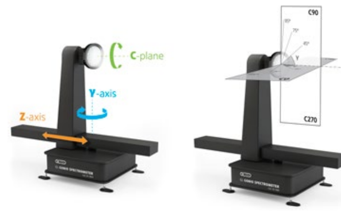
Fig. 3. Type C goniometer with three mechanized axes and schematic diagram of creating goniometric files for a typical luminaire.
